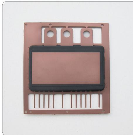
An integrated power module. These kind of customized modules, fully Ag-sintered, encapsulated and with double-sided cooling, are used for highly efficient inverters for EVs.
