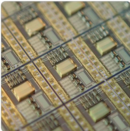
An optical multi-sensor wafer using Through Polymer Via (TPV) technology to create individual optical windows for each detector. This picture shows the wafer before singulation and assembly. Pictures above with courtesy of IC-Haus GmbH and Technical University of Delft.
