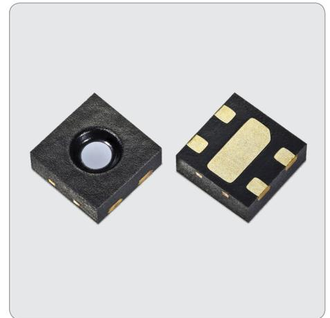
Humidity sensor on lead frame in QFN package. The top side shows an open (exposed) sensor area. The smallest window that can be designed with Film Assisted Molding is approximately  $\varnothing$  0.30 mm.
