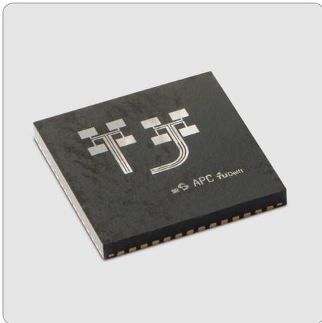
A 120 GHz transceiver package using Through Polymer Via (TPV) technology. TPV enables high density electrical or optical interconnects through your package. Picture above with courtesy of Silicon Radar GmbH and Technical University of Delft.
